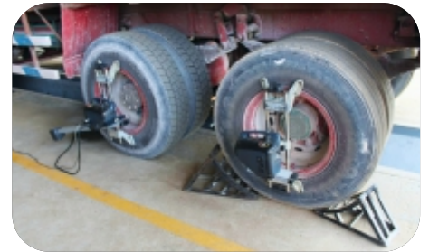
Run out operation for wheel alignment measurement
